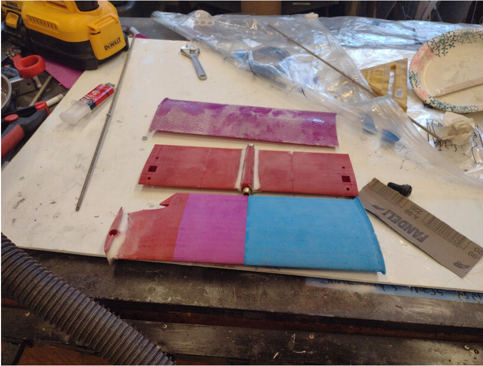
Figure 4.6 From top to bottom: finished aft mast, glued and faired aft foil, glued and faired forward mast. Notice the brass tube in the rear foil. This is a simple bearing that will support the drive shaft.
