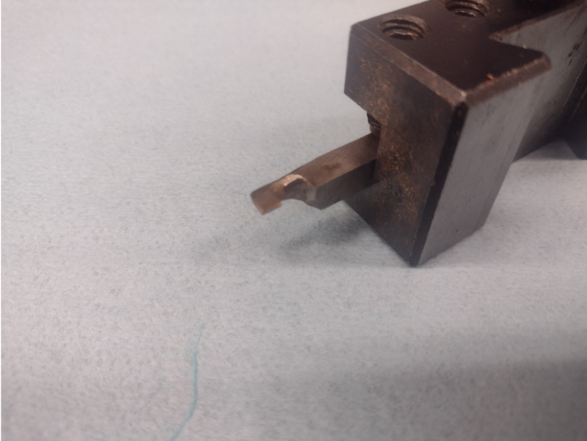
Figure 4.14 Pictured is the high speed steel tool clamped in a lathe toolpost. The cutting edge is relieved, and a substantial throat was cut behind the tool to allow the tool to reach into the bore of the O-ring gland.
