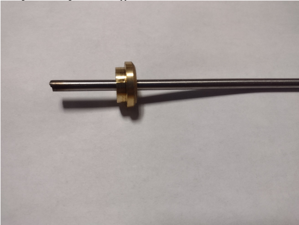
Figure 4.13 The 6mm stainless steel shaft rotates with little resistance in the brass cable gland. The brass is chosen for its low friction properties as a plain bearing, and for its resistance to corrosion in the presence of water.
