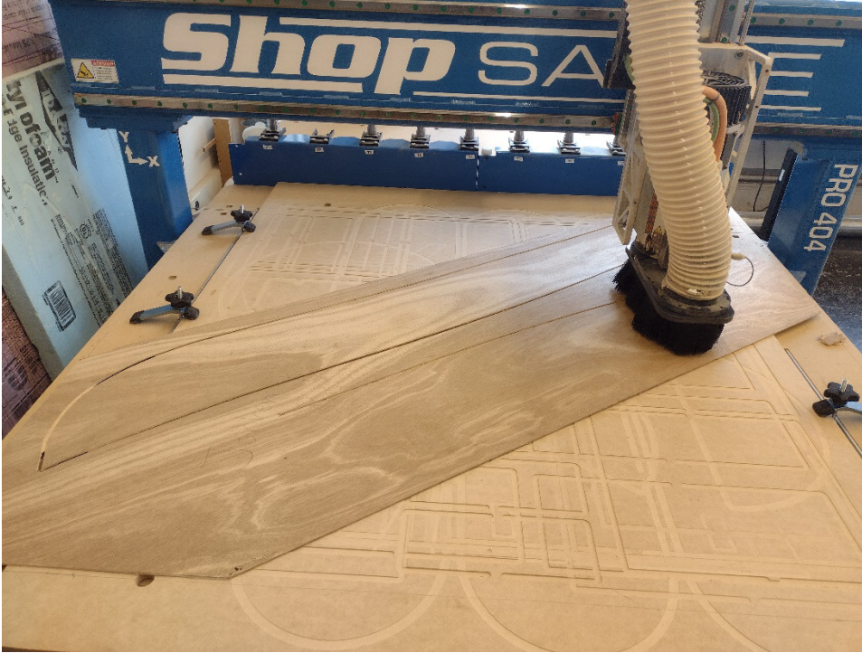
Figure 4.1 The 1/8in plywood is fixtured to spoilboard with small screws and cut with a ShopSabre CNC router.
