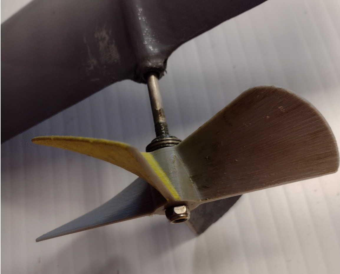
Figure 4.12 The end of the drive shaft is a stack of a locknut, prop, coupler, thrust washer, thrust bearing, thrust washer, and O-ring. Marine grease lubricates the shaft and O-ring and prevents the ingress of water.
