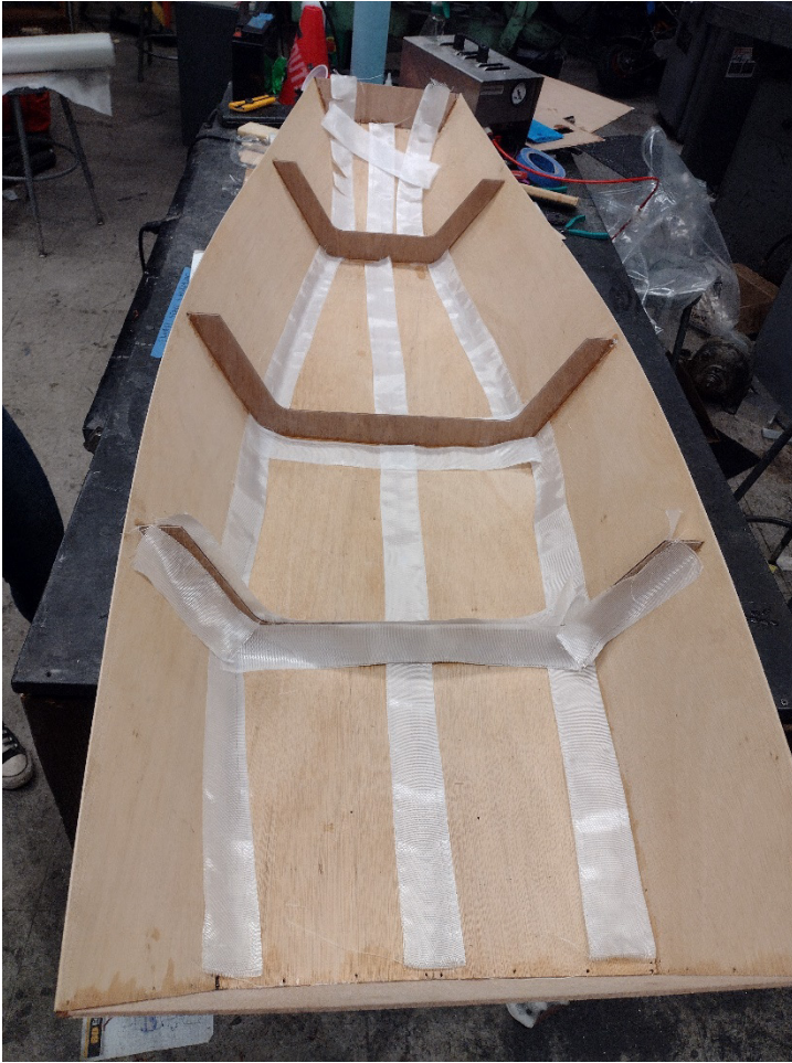
Figure 4.4 Fiberglass tape, visible in white, before being wetted out with epoxy. This tape will strengthen the joints.
