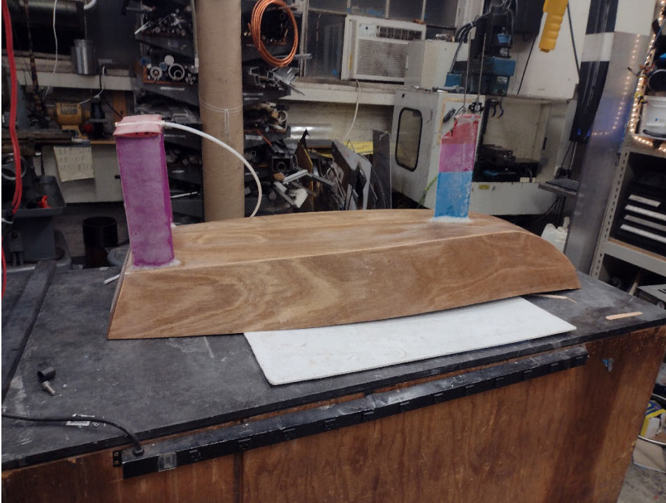
Figure 4.9 Note the PTFE tube attached to the rear foil. This will later penetrate the hull and forms a smooth, low friction liner in which the flex shaft will run. Finally, the hull was painted with Rust-Oleum Marine Topside paint to smooth the surface and improve waterproofing.
