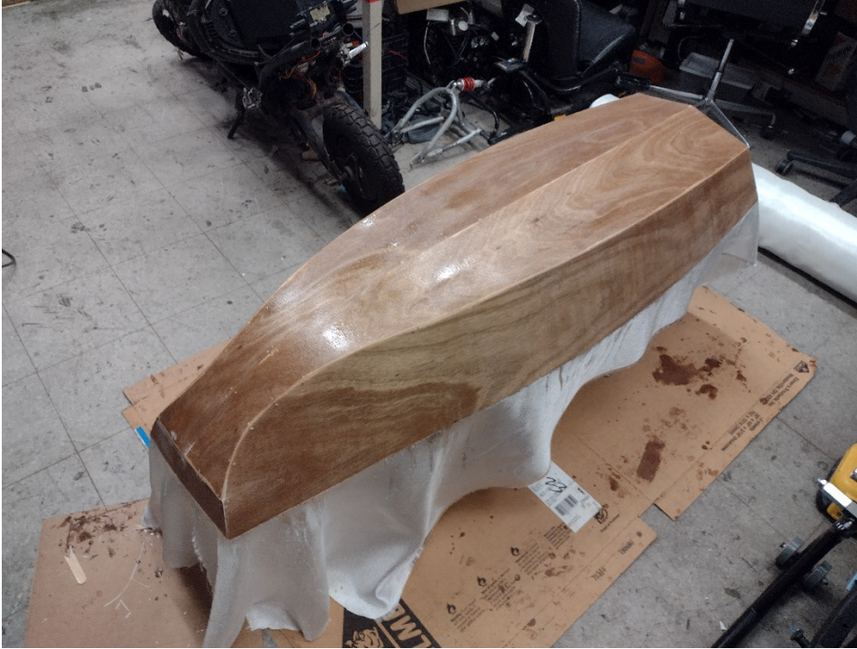
Figure 4.5 Where wetted out with epoxy, the fiberglass is clear.
